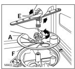
The dishwasher must not be used without filters. Incorrect repositioning and fitting of the filters will produce poor washing results.
